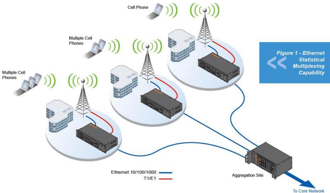
Figure 1 - Ethernet Statistical Multiplexing Capability
