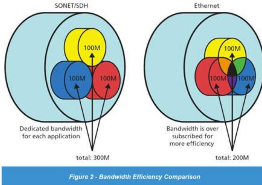
Ethernet is a connectionless packet technology that inherently supports statistical multiplexing. Ethernet-based backhaul transport can easily accommodate data increases with a much smaller incremental increase of backbone bandwidth through the proper use of over-subscription and statistical multiplexing. Industrial Ethernet layer 2 switches can be deployed in several applications to increase overall bandwidth efficiency including:
