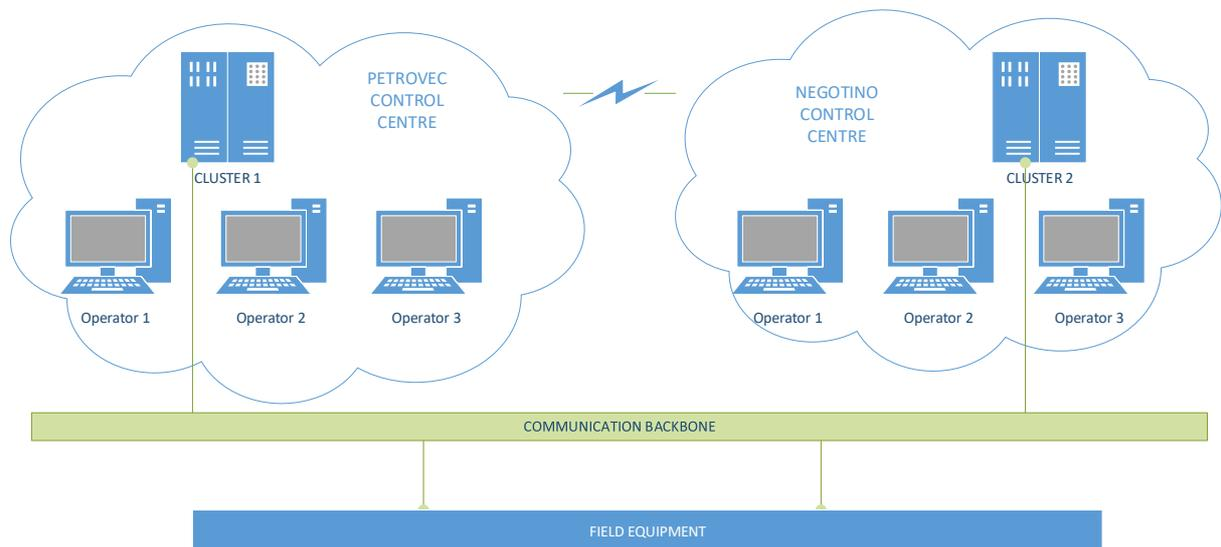
Redundancy should exist in two levels, local and remote. Local redundancy implies that within each control centre, servers are redundant (cluster mode). So, when a hardware or software component fails, automatically another hot-standby server within the same cluster takes over.
