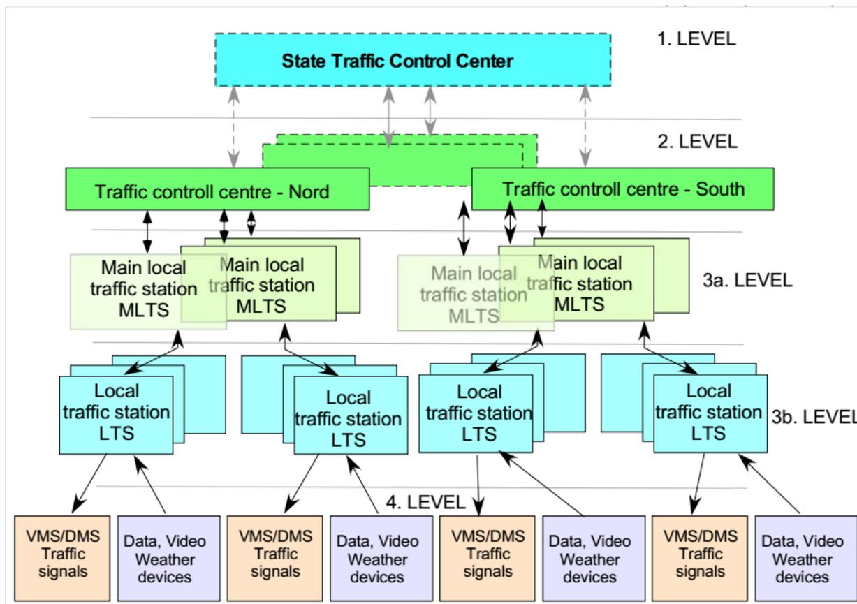
Since this is not our case, Level 3a and Level 3b devices (LTS & MLTS) can be omitted, providing less complexity and reliability (e.g. if one MLTS unit loses communication, everything below that unit will become unavailable), lower implementation cost (less CAPEX) and lower operational/maintenance cost (less OPEX). Field devices can be required to have an Ethernet interface that will enable the central system to communicate directly with them.
